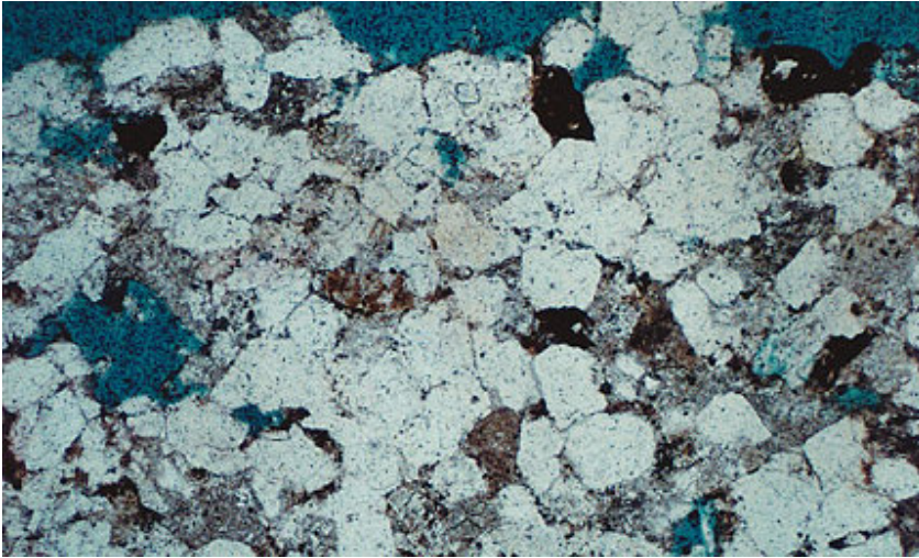
Fig.3b. Thin section Photo of a tight gas sandstone. The blue areas are pores. The pores are irregularly distributed through the reservoir and the porosity of the rock can be seen to be much less than the conventional reservoir.
